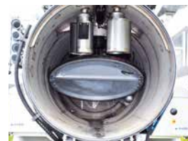
Hydraulically tiltable divider door
