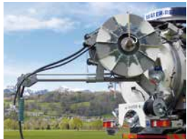
Jetting boom with KSA11 extension
