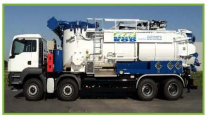
The trucks are highly versatile and may be used to collect and remove waste matter of any form, be it hazardous material, fine powdery material, grits, liquids or sludge.
